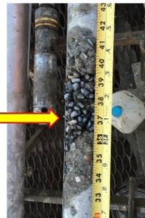
Anomalous low temperature detection investigated by coring resulting in detection of poor quality concrete.
